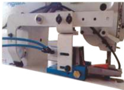
JZ-HTCM-L50 触动式切带装置 MANUAL CUTTING DEVICE
