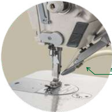
SIDE TYPE MMER ASSEMBLY 斜拉款剪线刀组
